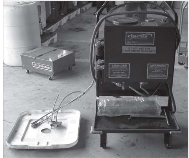
Fuel-motor oil blending system machine recycles waste motor oil.
