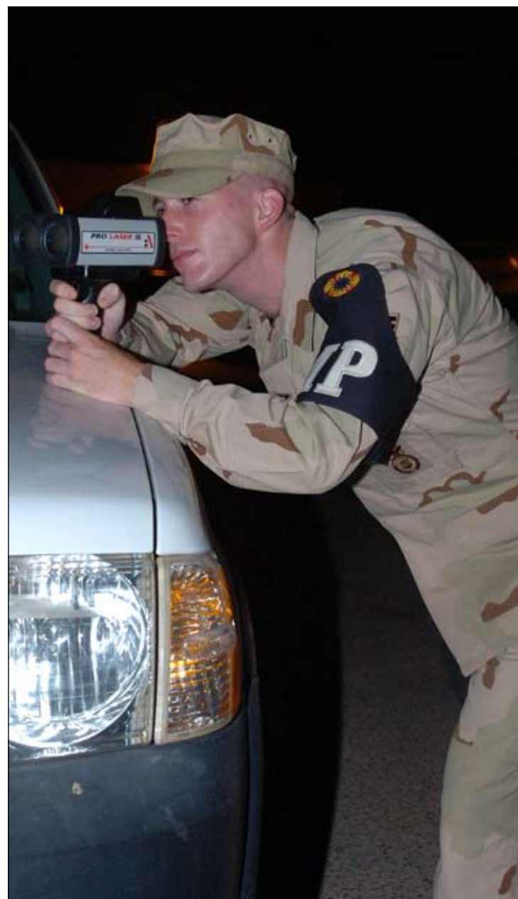
Air Force Staff Sgt. Edward B. Mann, desk sergeant and patrolman, 322nd Expeditionary Security Forces Squadron attached to the Provost Marshall's Office here, utilizes the new speed device, the Pro Laser III, outside his vehicle. The new device has been in use since May here and is more accurate than its predecessor. (Left) Air Force Staff Sgt. Edward B. Mann, takes a closer look at the reading on his new speed device, the Pro Laser III, outside his vehicle. The new device has been in use since May.
