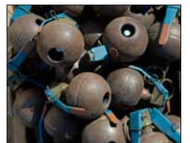
Training grenades, also referred to as "blue bodies," are used by SOI students to practice the throwing positions. The reusable grenade bodies are collected after being thrown and a new fuse mechanism is inserted. Cpl. Shawn Dickens/Chevron
