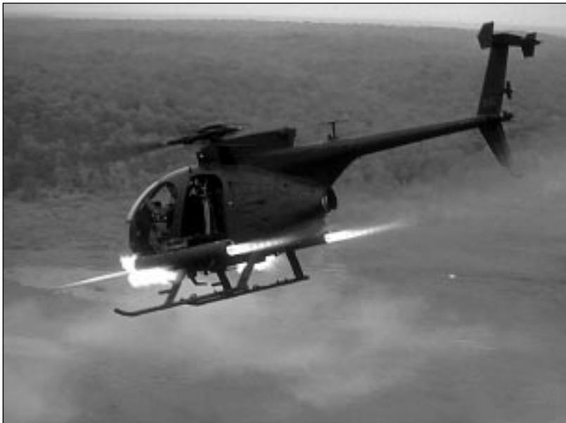
*The 160th SOAR's AH-6J helicopters are equipped with 2.75-inch rocket pods and can be equipped with a variety of other weapons.*
