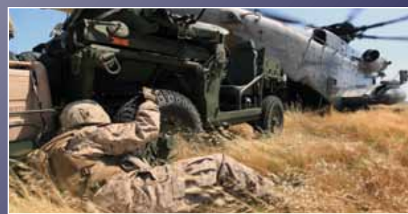
Lance Cpl. Romero Almanza from Battalion Landing Team 3/1, 11th Marine Expeditionary Unit, I Marine Expeditionary Force, based at Camp Pendleton, Calif., removes a roll cage from a light utility vehicle during an aerial transport exercise May 24. This is the first time that the Expeditionary Fire Support System has been loaded into an aircraft on the West Coast.
