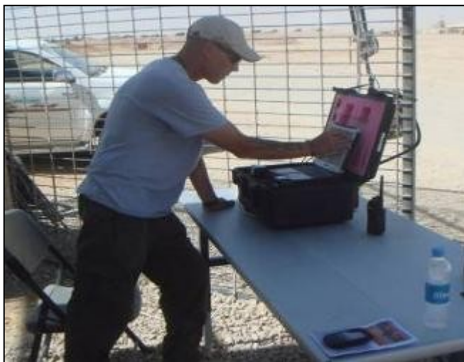
Left: Todd Patterson, unmanned aerial vehicle field service representative at Camp Leatherneck, field tests a new more compact T-Hawk system. The new compact carrying case was created for a unit to ease space constraints inside their tactical vehicle. The new case was constructed out of a pelican case and wire grates found in the Kandahar DLA Disposition Services Yard.
