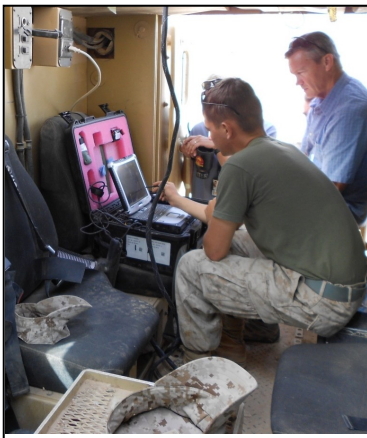
Left: Todd Patterson, unmanned aerial vehicle field service representative at Camp Leatherneck, field tests a new more compact T-Hawk system. The new compact carrying case was created for a unit to ease space constraints inside their tactical vehicle. The new case was constructed out of a pelican case and wire grates found in the Kandahar DLA Disposition Services Yard.
