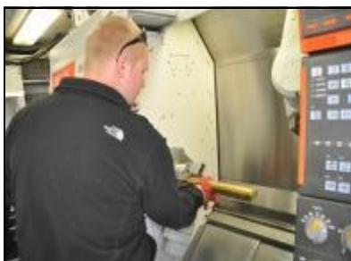
Left: Blake Brodeur, a machinist at the mobile parts hospital on Camp Leatherneck, from Anniston Ala., removes material from the five axis lathe at the parts hospital. The parts hospital is a rapid manufacturing system that can make needed replacement parts for most anything including trucks and aviation assets. They can also make custom parts and tools.
