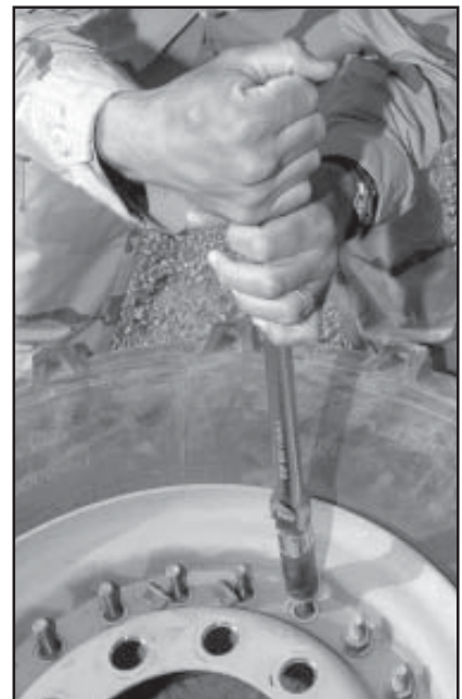
Without pneumatic equipment, the Troopers had to manually unscrew and tighten 19 bolts per tire. The grueling tasks can take up to five hours, however the crews were averaging two and a half hours per tire.
