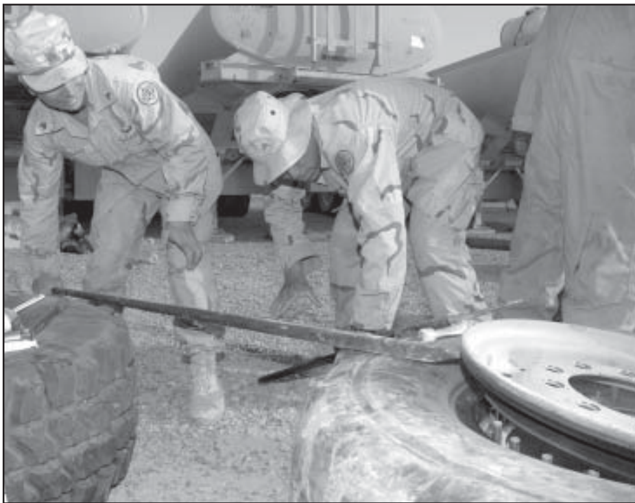
Sgt. David Sawyer, left, and Sgt. Christopher Ayala, team together to pop the rim off a worn tire. The two petroleum supply specialists, assigned to Suppy & Transportation Troop, Support Squadron, replaced several tires during preventative maintenance checks and services at Camp Striker, Iraq.
