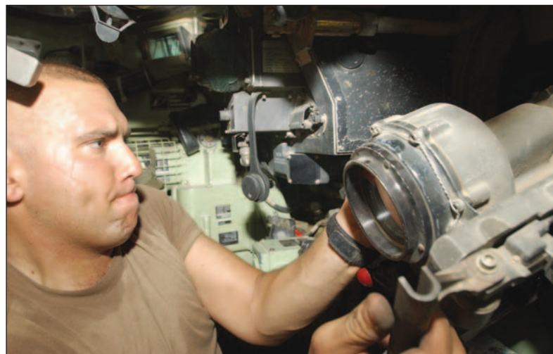
Spc. Markus Bennett removes the weapon breech from the turret on a Bradley fighting vehicle being serviced.
