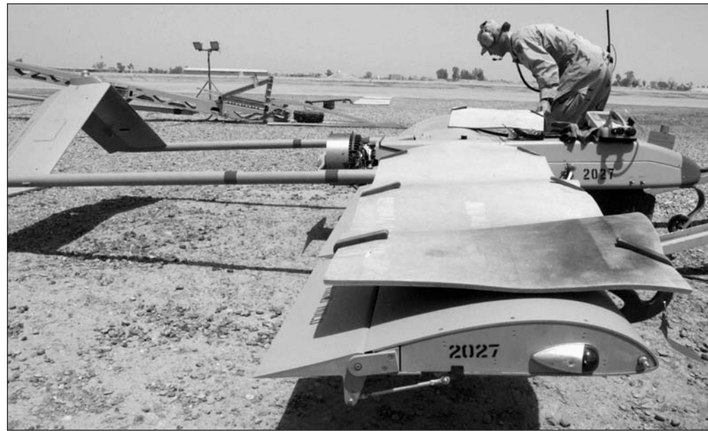
Spc. Joshua Eldridge, assigned to the 3rd Infantry Division’s 1st Platoon, Tactical Unmanned Aerial Vehicle Company, Special Troops Battalion, conducts a pre-flight inspection of a Shadow 200 TUAV.
