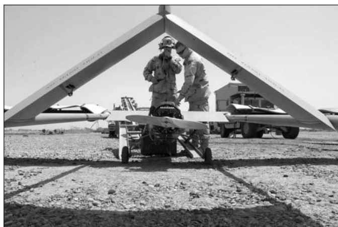
Spc. Joshua Eldridge, a Titusville, Fla., native, and Spc. Sean Davis, from St. Petersburg, Fla., conduct a preflight inspection of a Shadow 200 Tactical Unmanned Aerial Vehicle prior to its launch. Both Soldiers are assigned to the 3rd Infantry Division’s TUAV Co., Special Troops Bn.
