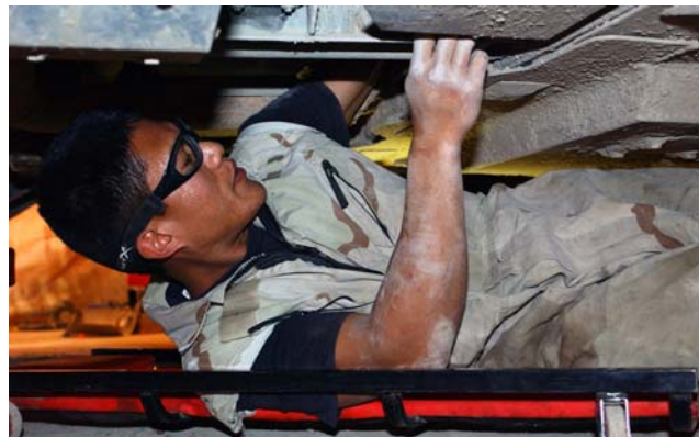
Staff Sgt. Shawn Reed finishes putting on a wheel after replacing the brakes on a forklift. (Photos by Master Sgt. Jon Hanson)
