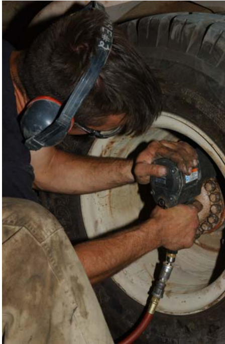
Staff Sgt. Shawn Reed finishes putting on a wheel after replacing the brakes on a forklift. (Photos by Master Sgt. Jon Hanson)
