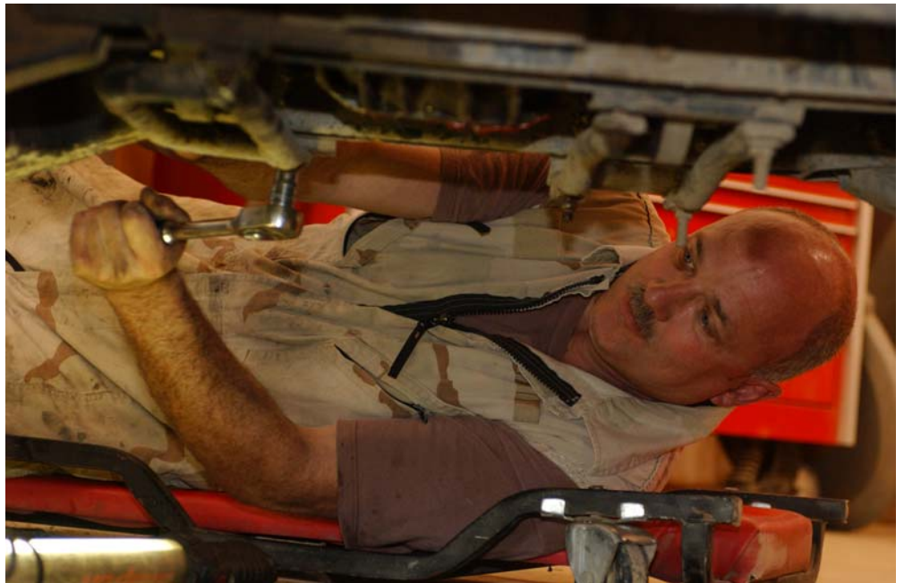
Staff Sgt. Rick Adams tightens a Humvee's front brake support brackets.
