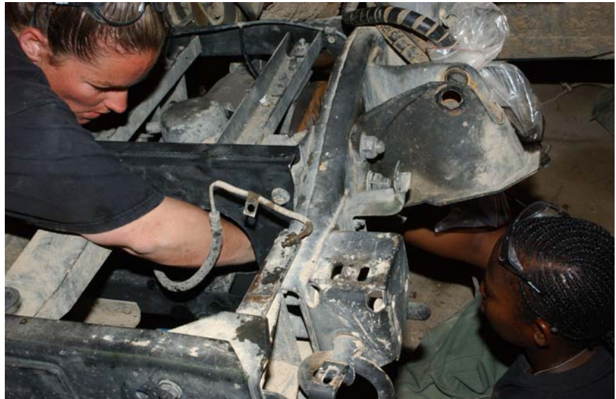
Above: SSgt. Shane Chandler (left) and Senior Airman Kimberly Louis install a brake assembly on a Humvee. Left: SSgt. Nicomedes Macadaan rewires a vehicle's transmission computer wires.
