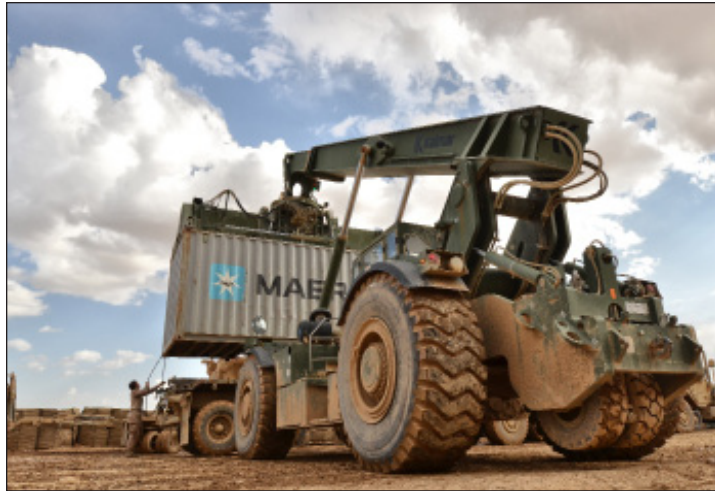
A rough-terrain container handler off-loads a shipping container from an Alpha Company, Combat Logistics Battalion 4, 1st Marine Logistics Group (Forward), Logistics Vehicle System Replacement at Forward Operating Base Edinburgh, April 22. The shipping container was delivered to the FOB during a six-day combat logistics patrol.
