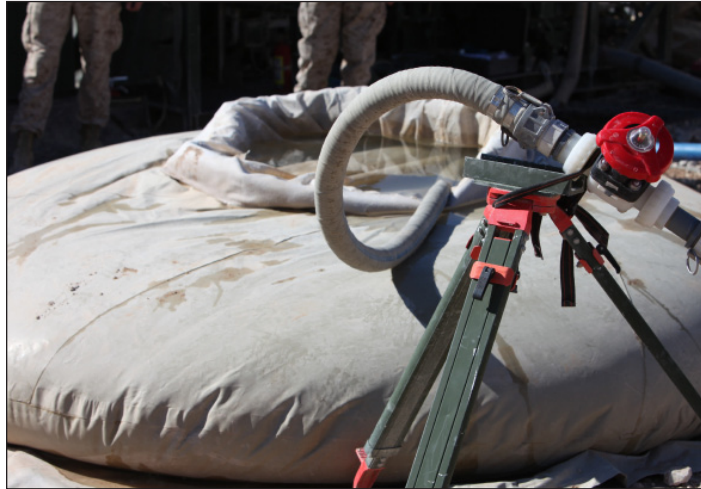
After retrieving water from the Helmand River in Afghanistan, the water point team from Support Company, 9th Engineer Support Battalion, 1st Marine Logistics Group (Forward) transfers water from the trucks to a water bladder to await purification at Forward Operating Base Whitehouse.
