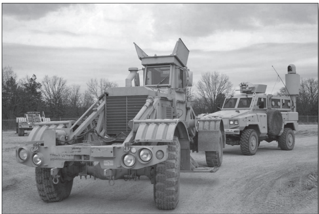
A Husky (front) and an RG-31 set off on a route clearance patrol.
