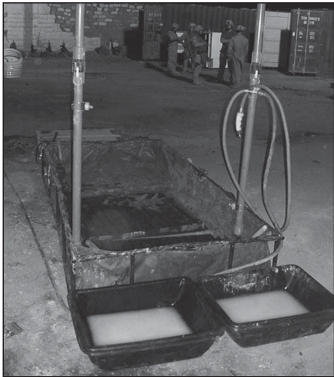
Decontamination shower used by personnel exiting the hot area
