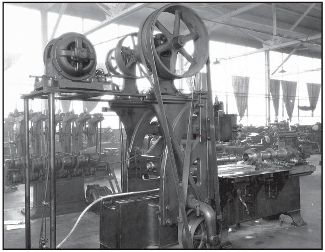
Mortar barrels are rifled in McBride's machine shop, Edgewood Arsenal, 1924.
