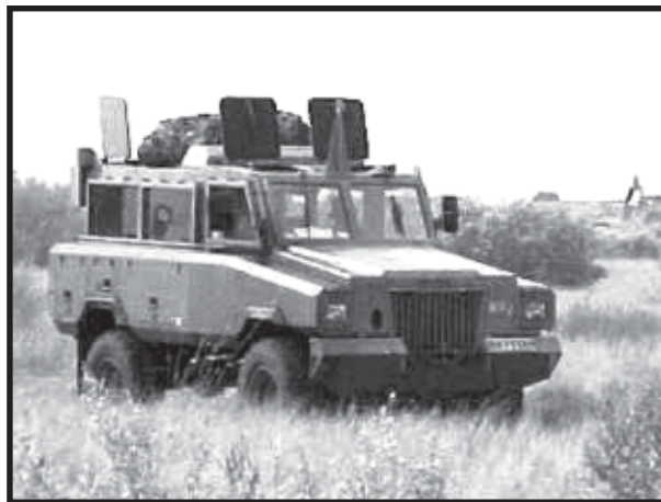
The Mamba is the primary vehicle of the South African army military police.
