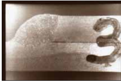
This is an example of a test piece. It was for testing a patch repair of a diffuser case.
