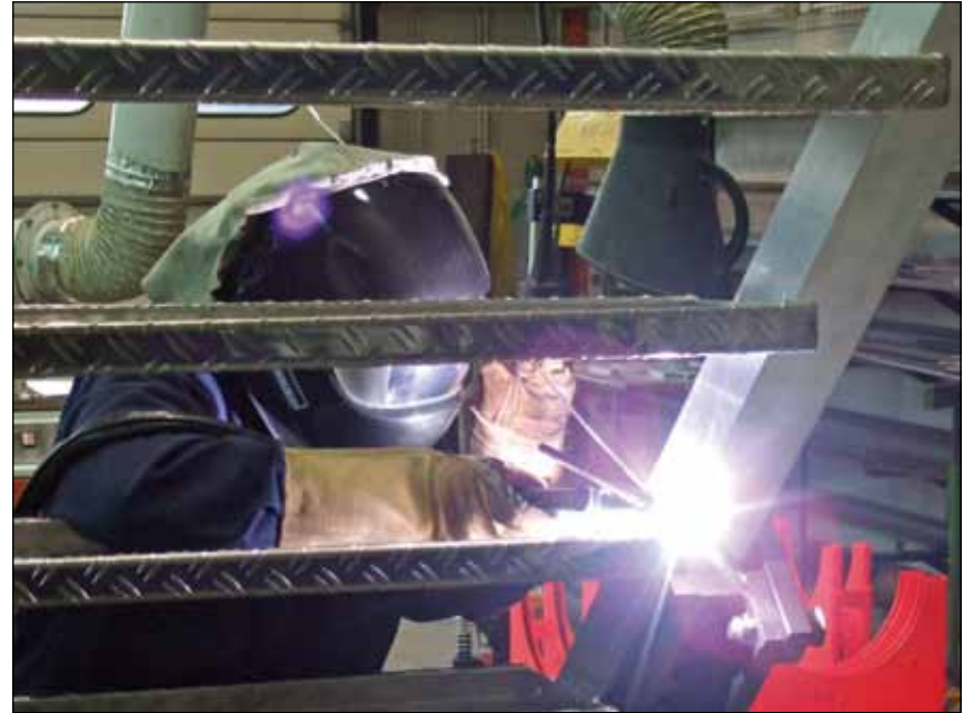
This is a stairway that was designed and manufactured/welded by welding shop. It's one example for things that welding shop manufactured for other shops and section.
