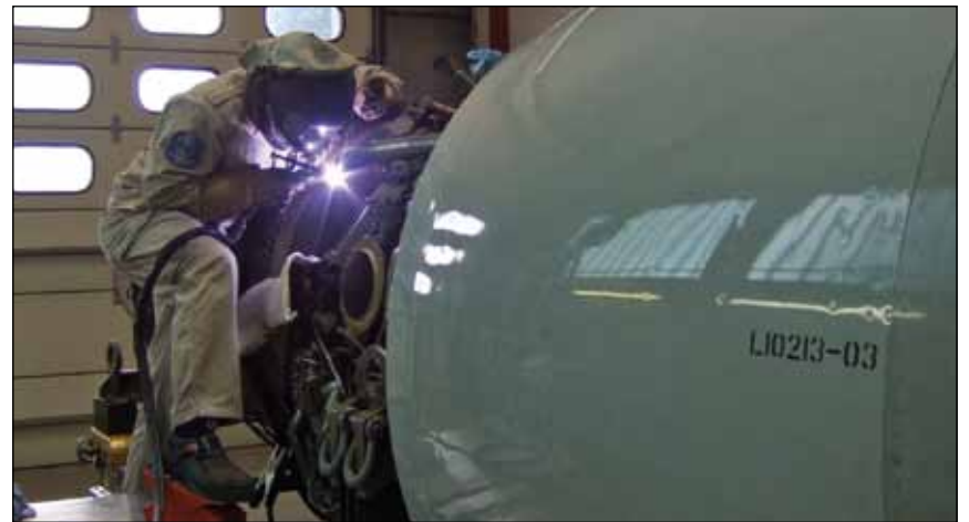
An aircraft welder performs a weld on a cracked diffuser case.
