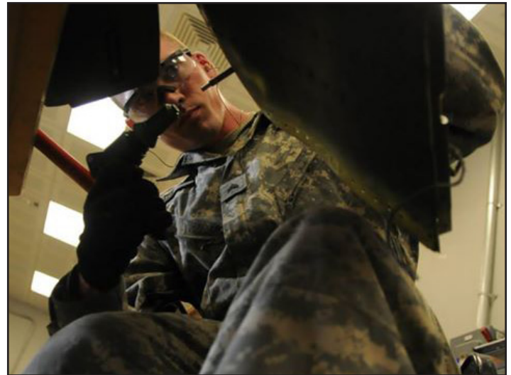
BAGRAM AIRFIELD, Afghanistan - Sgt. Mitchell Pace, an aircraft structural repairer assigned to the Airframe Shop, B Company, 277th Aviation Support Battalion, Task Force Phoenix, 10th Combat Aviation Brigade, lines up a rivet with a rivet puller as he replaces a brace on a CH-47 Chinook helicopter platform here Sept. 24, 2013. (Photo by Staff Sgt. Todd Pouliot, 10th Combat Aviation Brigade)
