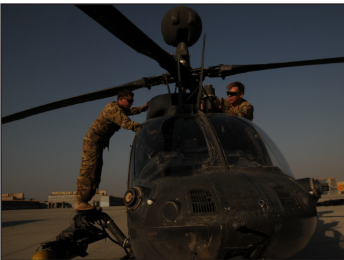
BAGRAM AIRFIELD, Afghanistan - From left, Sgt. Andrew Gage, an OH-58 Kiowa Warrior helicopter crew chief; and Sgt. 1st Class Corey Shelton, a Kiowa Warrior platoon sergeant; reinstalls the forward cowling during a preventative phase maintenance service on a Kiowa Warrior here Oct. 7, 2013. (Photo by Staff Sgt. Todd Pouliot, 10th Combat Aviation Brigade)
