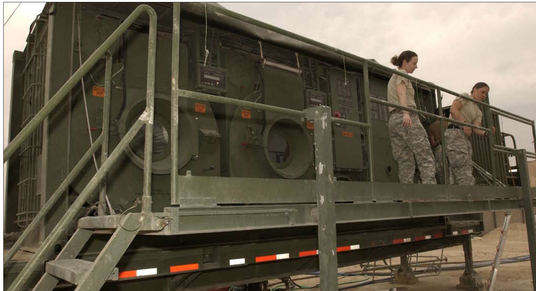
The Laundry Automated Draining System combines the capabilities of washers and dryers in one machine.
