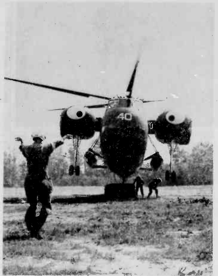
MY, WHAT BIG EYES! —And a strong back, too! Ground crewmen direct an HR25 into position to airlift a 6,000-pound rolling container of fuel at the Landing Force Development Center at Quantico.
