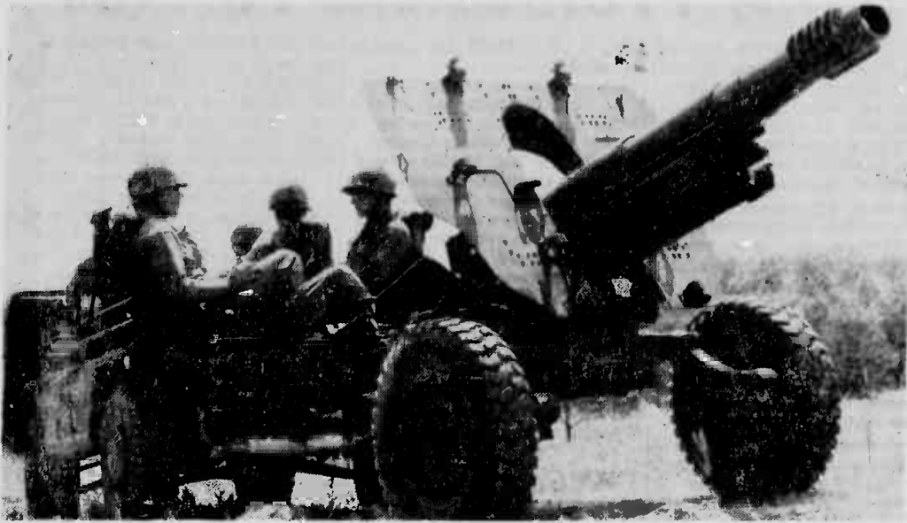
A COMPACT FOREIGN MODEL —This Marine gun crew, riding on a "convertible mule," tows an Italian-developed 105mm Pack Howitzer to an area for practice firing. The howitzer weighs only 2,860 pounds and breaks down into 16 component parts which can be man-carried.
