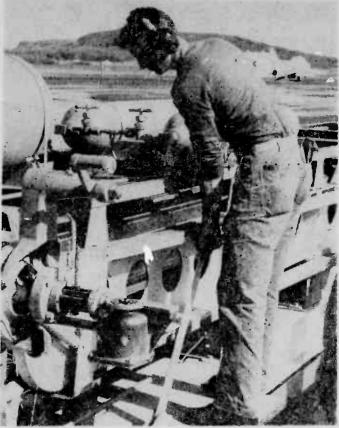
PRESSURE ADJUSTER - Once the pilot radios in his aircraft type and fuel capacity, this man sets the pressure on the arresting gear.
