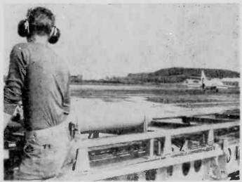
A SUCCESSFUL "CATCH" - This F9F finds itself caught as a crew man checks the mechanism to make sure everything is functioning perfectly. If the pilot should miss the first hook he has a second cable to rely on.
