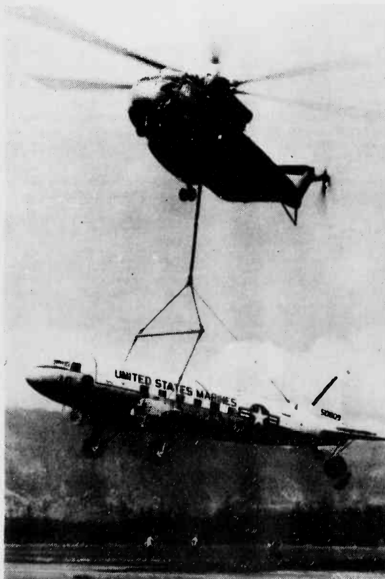
A show of aerial power— 8,000 pounds of airplane fuselage being lifted by a CH-53D.
