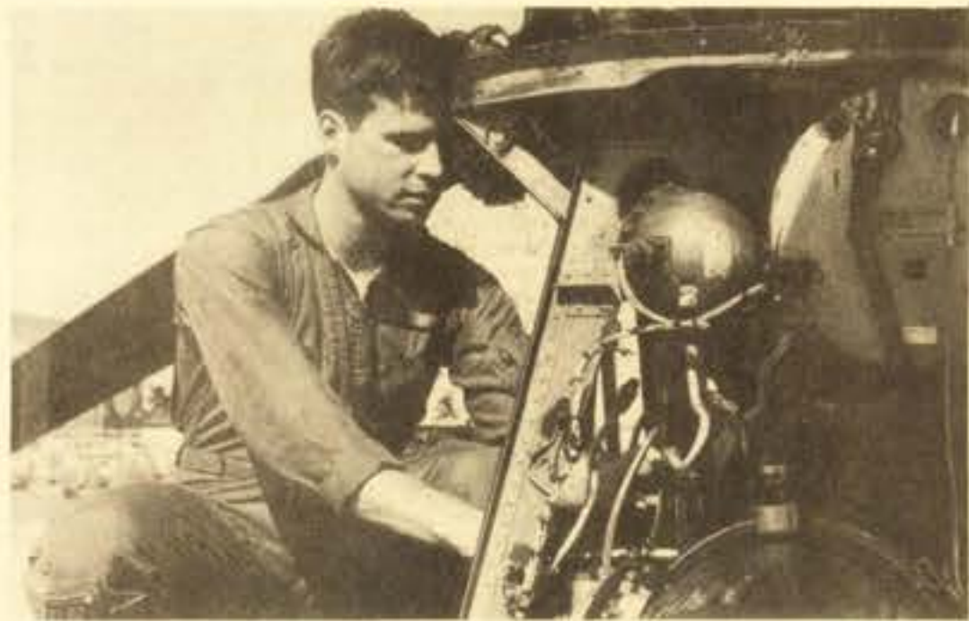
DOUBLE CHECKING — Corporal Christopher R. Miller, Marine Medium Helicopter Squadron-265, checks the strut (nosewheel) of his aircraft during a
