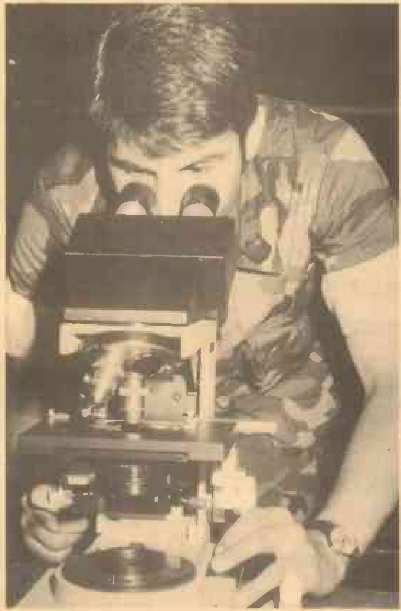
BLOOD COUNT — Hospital Corpsman 3rd Class Quincy Fletcher, lab technician, prepares a hemoglobin sample for blood count on a spectrophotometer (specimen light meter) (Photo by Cpl. J.T. Clark)
