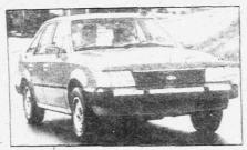
comes from its 1949cc single overhead-cam engine with I-TEC (Isuzu Total Electronic Control). an advanced fuel injection system. Standard transmission is a 5-speed manual with over-drive: a 4-speed automatic transmission with an electronically controlled overdrive 4th gear is optional.
