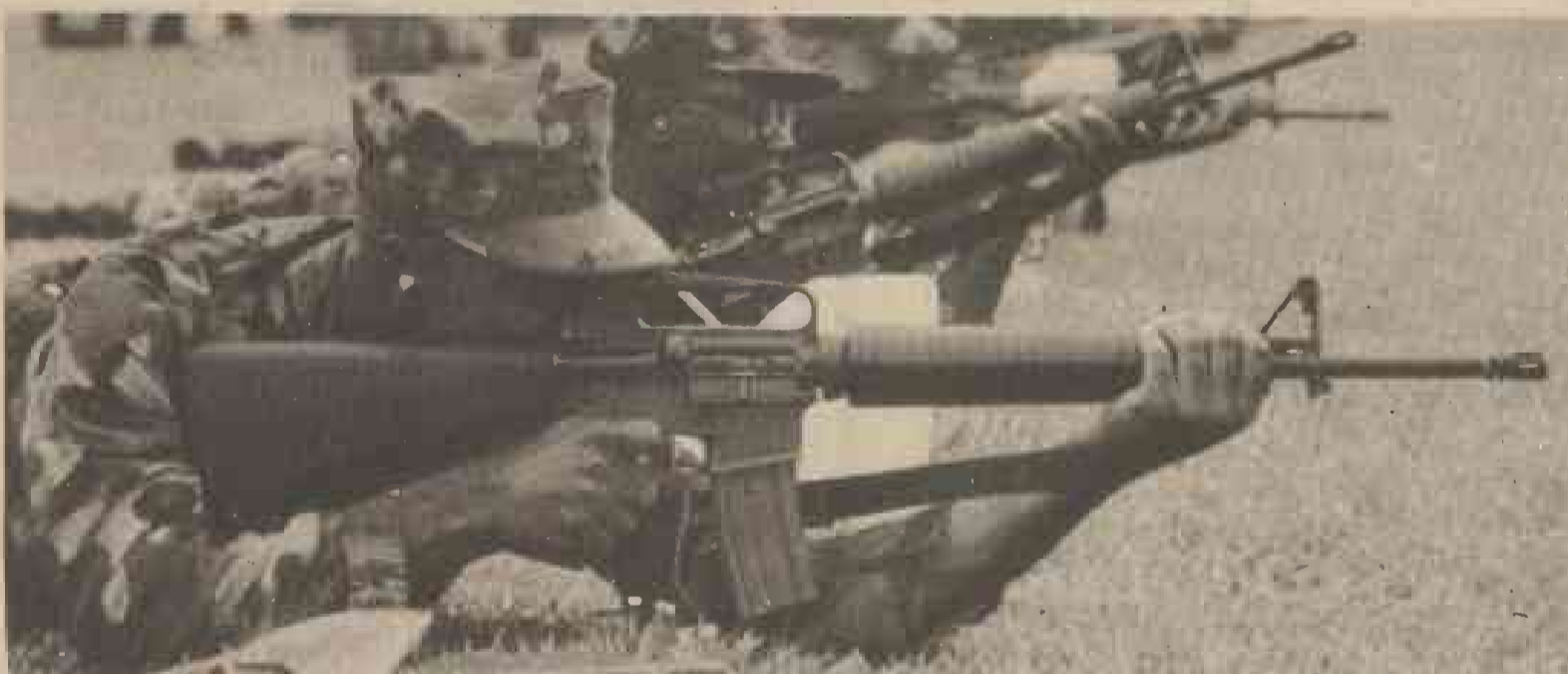
The M-16A2 service rifle features improved sight adjustments and a trigger mechanism with three distinct pulls.
