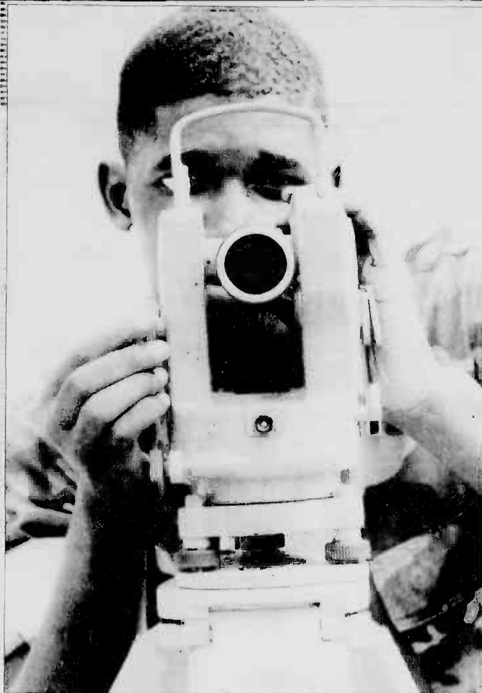
L.Cpl. Harry Doe, a surveyor, sights a theodolite on the PADS to plot a position.
