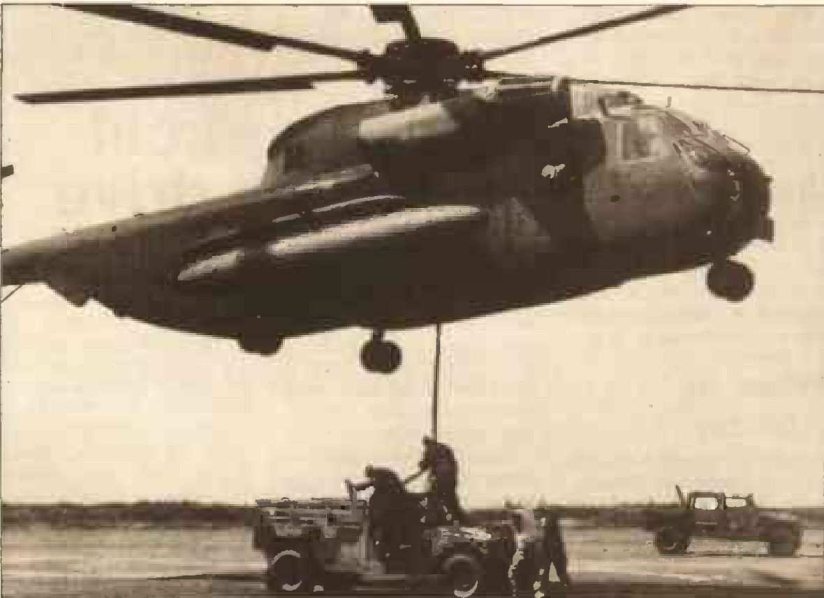
Marines from BSSG-1's 1st Landing Support Platoon attach a tactical vehicle to a CH-53's pendant during the Eagle Provider exercise.
