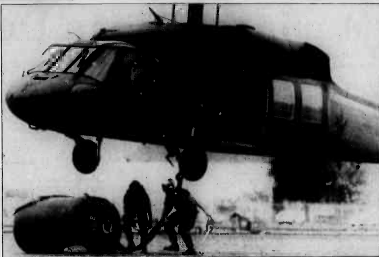
A pair of Landing Support Platoon Marines attach a 500-gallon fuel bladder to an Army helicopter. Helicopter Suspension Teams are only one of many specialties represented within Landing Support Co. A, 3d Landing Support Bn. here.
