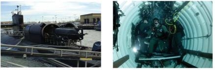
MK VIII MOD SEAL Delivery Vehicle and Dry Deck Shelter
