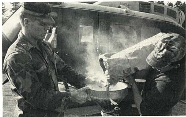
The M-5 gas unit is loaded with 100 lbs. of talcum powder for the simulated attack. (Photo by Sgt. Don Green)
