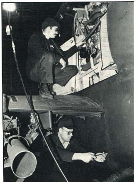
SSgt. Jim Bullion, top, inspects a Cobra transmission as SSgt. Lee Hayes fastens an inspection panel.
