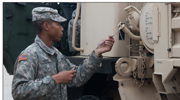
Above Pfc. Xavier Finger, wheeled vehicle mechanic, Headquarters and Headquarters Battalion, 1st Infantry Division Artillery, 1st Infantry Division, checks fluid levels on a M1078 Light Medium Tactical Vehicle, Oct. 5, 2015, at the unit's motor pool on Fort Riley, Kansas. (U.S. Army photo by Staff Sgt. Jerry Griffis)
