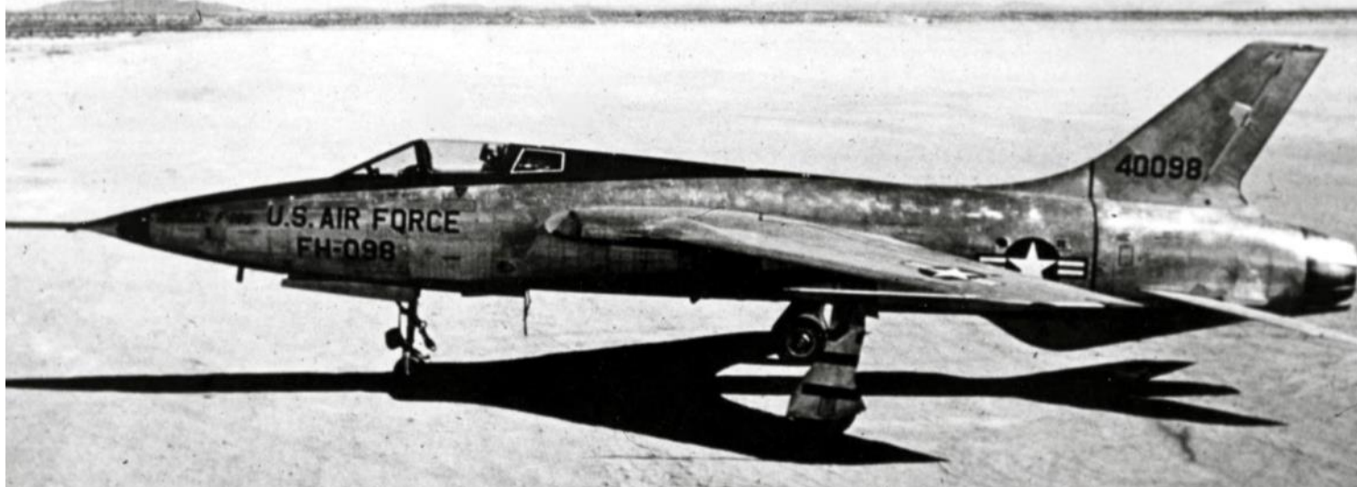
The first YF-105A Thunderchief prototype is shown at Edwards AFB; note the similarity to the RF-84F Thunderstreak in general configuration. (Republic Aviation/USAF photo.)
