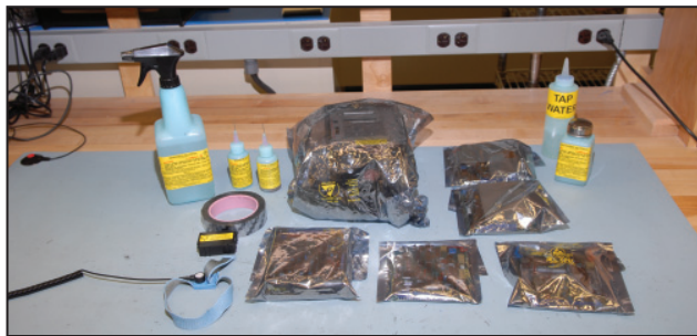
Various AN/ARC-186 Receiver/Transmitter components are stored in ESD safe bags prior to inspection. Other ESD-approved equipment used at the work bench include a wrist strap and bottles for tap water and alcohol.
