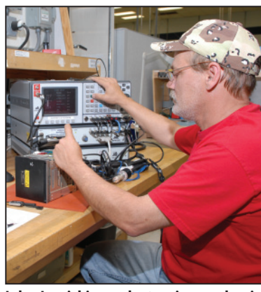
John Lywiski, an electronics mechanic, uses an automated test set to adjust an AN/ARC-186 Receiver/Transmitter during a final test procedure.
