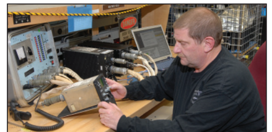
Robert Dusseault, an electronics mechanic, performs a self-diagnostic test on an ARC/220 High Frequency Receiver/Transmitter
