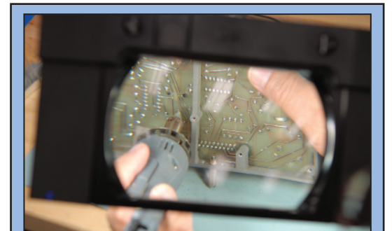
Frank Gervasi, an electronics intern, replaces a capacitor on a receiver subassembly circuit card for the Air Force's AN/ARC-186 Receiver/Transmitter.
