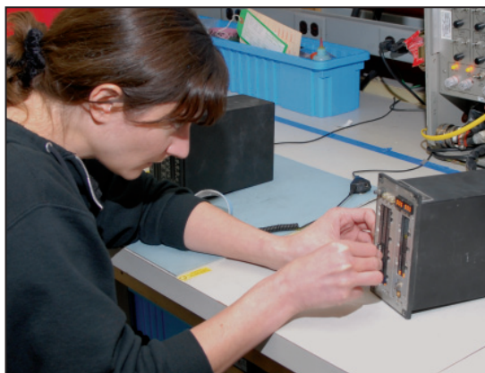
Angela Dalmas, a SCEP student, replaces a lamp module on a Pilot Display Unit, which is part of the UH-60 Black Hawk's Vertical Instrument Display System.
