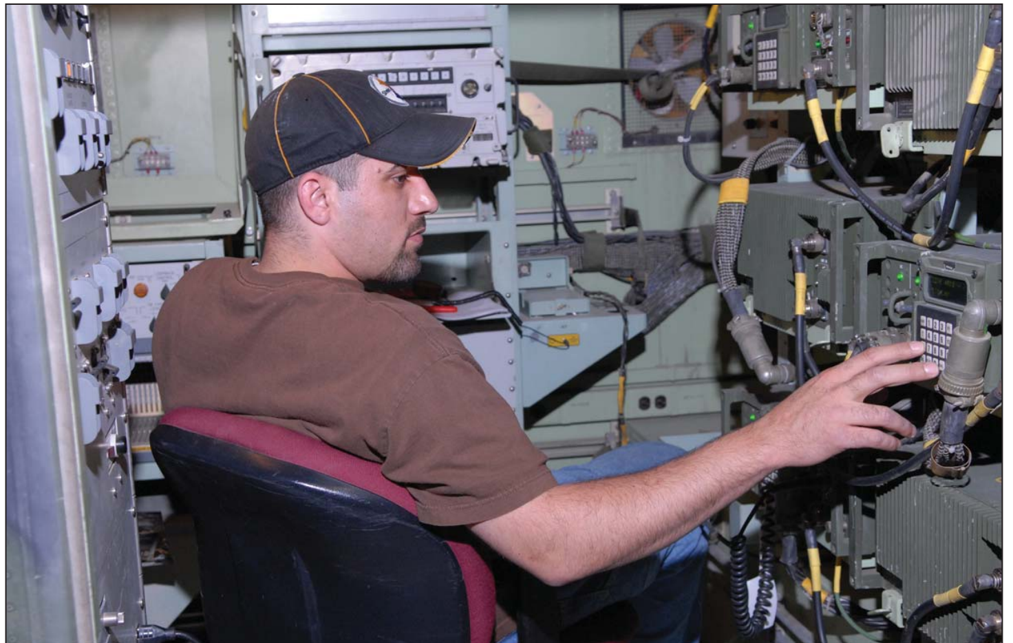
Richard Robinson, an electronics worker in the DGM/MSE Branch, tests the AN/GRC-245 HCLOS radios during the pre-test part of the AN/TRC-190 Reset process. (Photo by Tony Medici)
