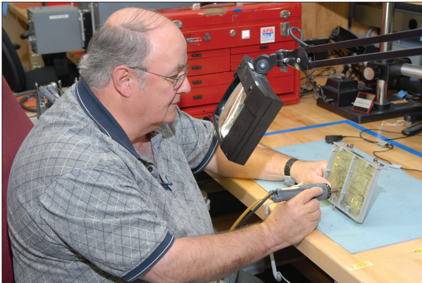
Dale Stine, an electronics mechanic, de-solders an electronic component on an A1 circuit card assembly as part of the SH-60 Navy Sea Hawk "Tip to Tail" program.
