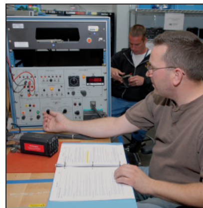
James Filipowich, an electronics worker, runs a final test procedure on a UH-60 Black Hawk's C-10998 Mode Selector Panel.
