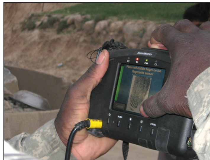
A Soldier demonstrates how to record a person's fingerprint using the Handheld Interagency Identification Detection Equipment (HIIDE). (U.S. Army photo)
