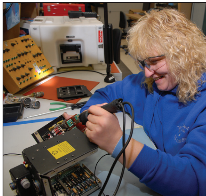
Christine Harmady, an electronics mechanic, changes a faulty switch on a C-10909 Stabilator Flight Control Panel used in a Black Hawk.
