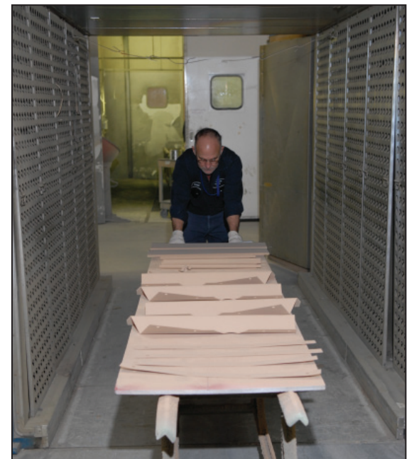
Donald Brown, painter's helper, places a rack of just-painted parts in an oven for drying.
