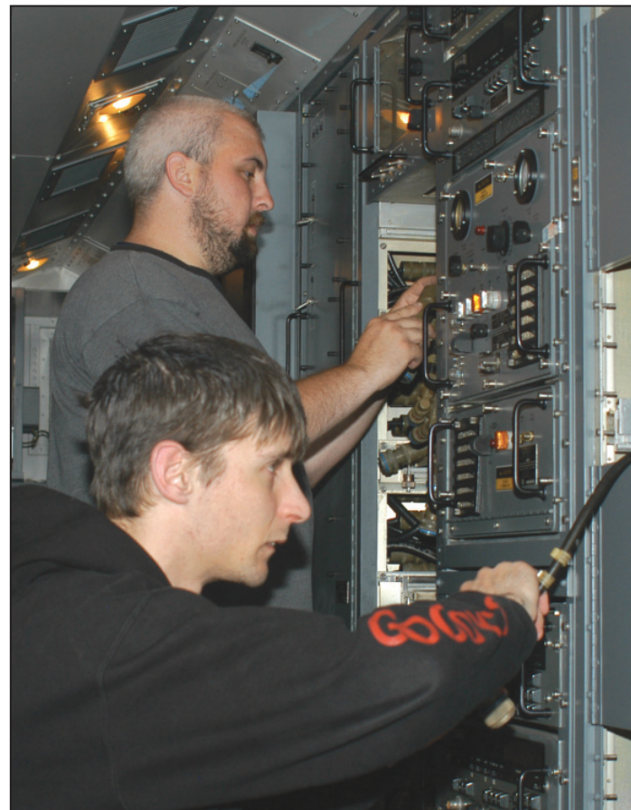
Thomas Lohman (seated) and Kenneth Blanchard prepare an AN/TYQ-23 Tactical Air Operations Module for final inspection. Lohman and Blanchard are electronics workers in the Command, Control and Computer/Avionics Systems Directorate. (Photo by Anthony Ricchiazzi)
