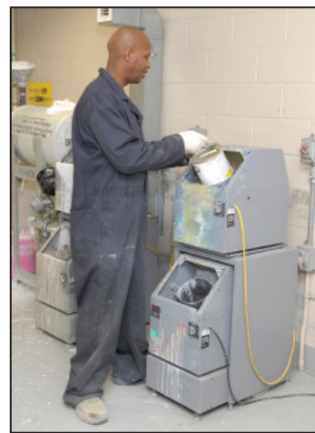
Tyrone Littles, painter, prepares CARC paint using a paint shaker.
