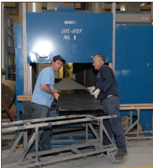
Darren Stout (left) and Donald Brown, painter helpers, process parts through a conveyor oven.
