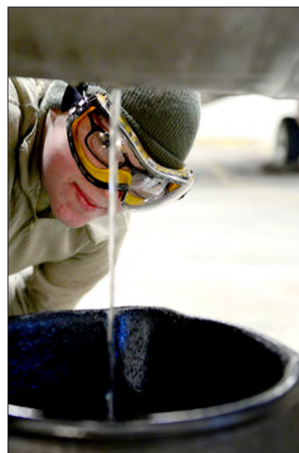
U.S. Air Force Senior Airman Jerri Addison, a 354th Aircraft Maintenance Squadron crew chief, watches fuel empty from an F-16 Fighting Falcon fuel tank into a bucket Nov. 22, at Eielson Air Force Base Alaska. The fuel was emptied into buckets and moved to another tank to be reused later. (Photo by Airman Eric M. Fisher, 354th Fighter Wing Public Affairs)
