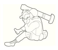
Javelin – The first "fire-and-forget" shoulder-fired antitank missile now fielded to the U.S. Army and U.S. Marine Corps, replacing Dragon. Javelin's unique topattack flight mode, superior self-guiding tracking system and advanced warhead design allows it to defeat all known tanks out to ranges of 2500m.
