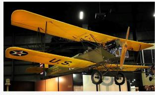
Above: The 119th Observation Squadron's original complement of aircraft included the Consolidated Aircraft PT-1 primary trainer. As shown in the photo of one of the remaining three PT-1s in existence, the engine cowling was often left off to both aid in cooling and provide easy maintenance access. (NMUSAF photo)
