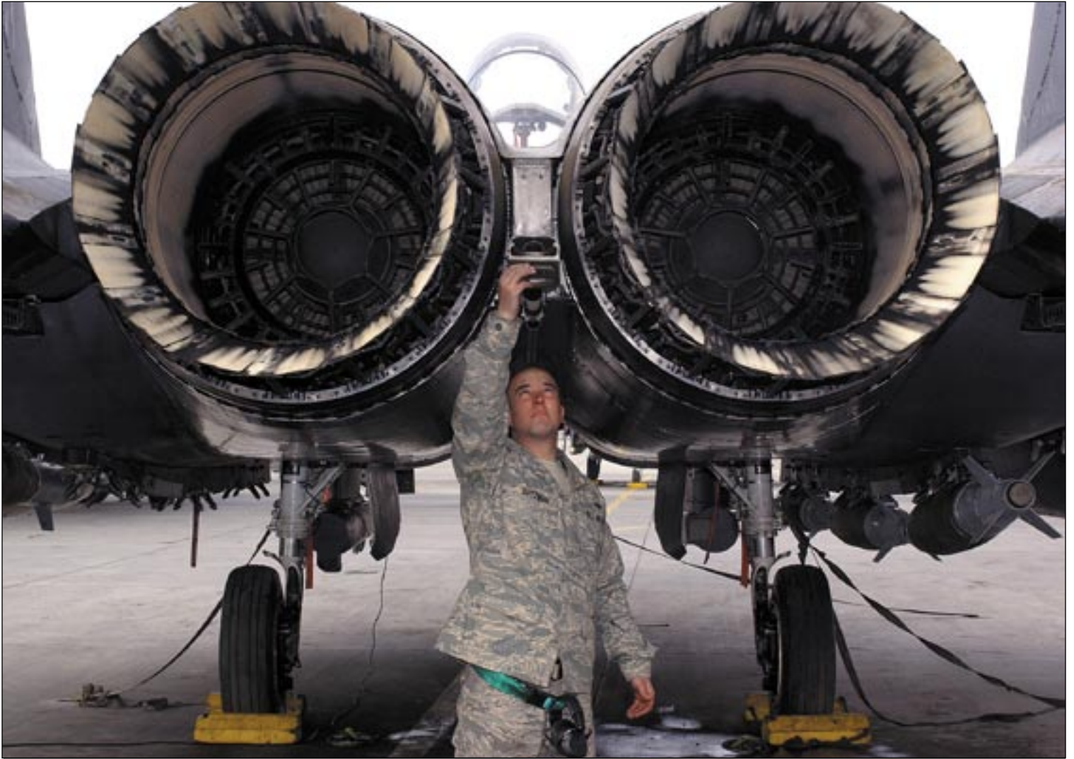
Airman 1st Class Erik Botzman, 455th Expeditionary Aircraft Maintenance Squadron tactical aircraft maintenance crew chief, checks the tail hook on an F-15E before a combat sortie. Botzman's home unit is the 335th Aircraft Maintenance Squadron at Seymour Johnson Air Force Base, N.C. (U.S. Air Force photo by Master Sgt. Demetrius Lester)
