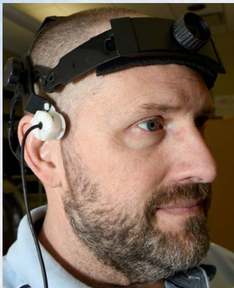
Jeffrey Howard, a general health scientist and epidemiologist at the U.S. Army Institute of Surgical Research and primary investigator, uses a transcranial Doppler technology called the Neurovascular Complexity Index to evaluate a new algorithm that measures cerebral blood flow velocity. (Photo by Steve Galvan)
