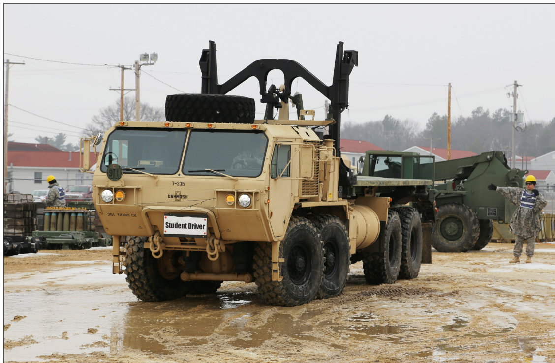
Students with the 13th Battalion, 100th Regiment's 89B10 Ammunition Supply Course operate an M1075A1 Palletized Load System truck during course operations Feb. 28 at Fort McCoy.
