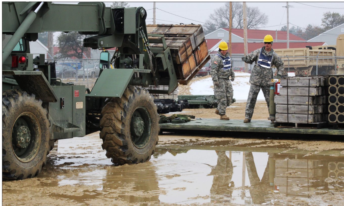
Students with the 13th Battalion, 100th Regiment's 89B10 Ammunition Supply Course load ammunition pallets using an All-Terrain Lifter, Army System forklift during course operations Feb. 28 at Fort McCoy.
