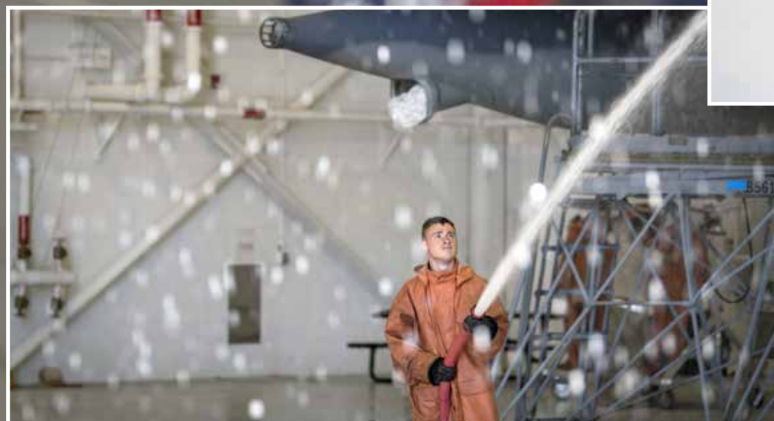
U.S. Air Force photo by Airman 1st Class Eugene Oliver Senior Airman Aaron Brewer, 71st Aircraft Maintenance Unit crew chief, uses a power washer to clean an HC-130J Combat King II, May 7, 2018, at Moody Air Force Base, Ga. Upon return from a deployment or every 180 days, HC-130s are thoroughly cleaned and inspected as part of routine upkeep and to ensure components are in working condition.
