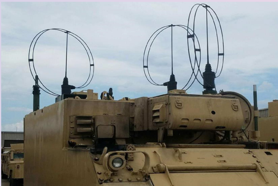
The near vertical incident skywave loop antennae installed on M1068 Battalion Fire Direction Center. (Courtesy photo)
