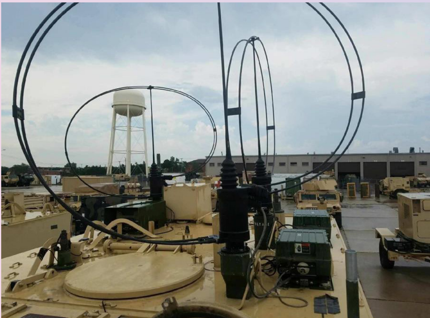
The near vertical incident skywave loop antennae installed on the battalion fire direction center. (Courtesy photo)
