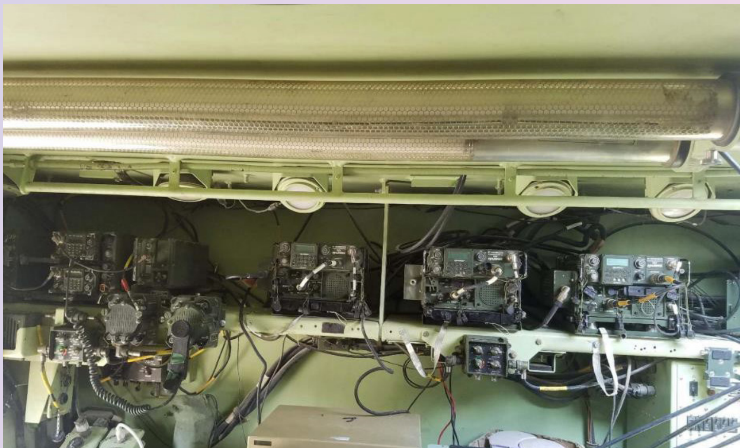
Parallel construct of three high-frequency radios (right) and standard frequency modulation voice and digital (left). (Courtesy photo)
