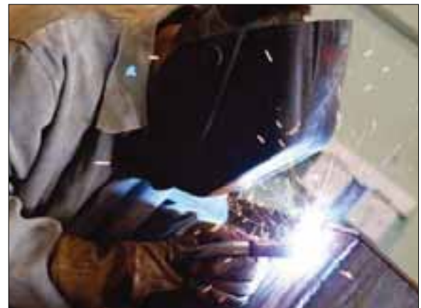
U.S. Army photo by Spc. Kiyoshi C. Freeman Spc. Jared L. Mauer, of Miami, Okla., uses a MIG welder to fabricate a lockbox for sensitive items at the “Skunk Werks” welding shop at Joint Base Balad, Iraq, April 9. While the shop was once well-known for up-armor vehicles, now the “Skunk Werks” occupies most of its time making more routine items, such as retention rings and this lockbox.
