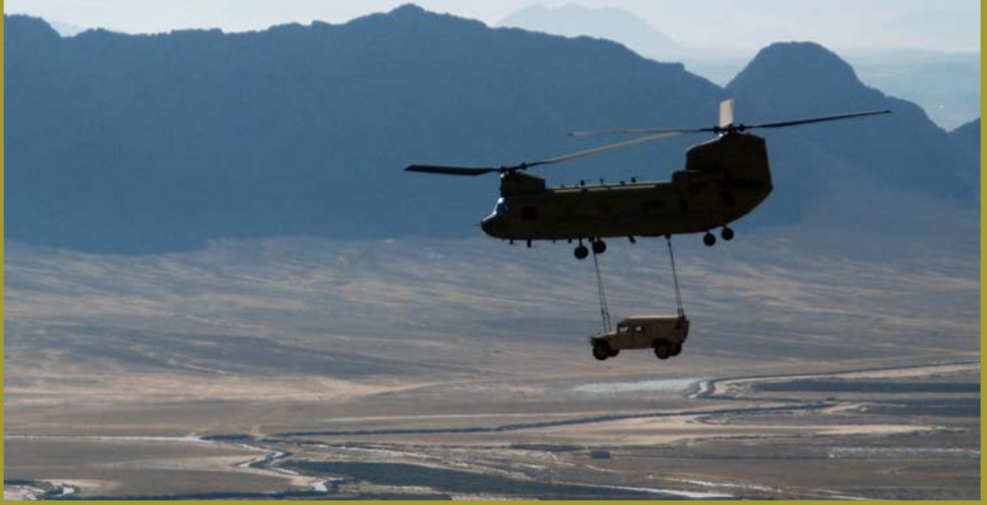
(Above) US Army CH-47F Chinook helicopter from Company B, 3rd Battalion, 82nd Aviation Regiment sling-loading a high mobility multipurpose wheeled vehicle (HMMWV) over Kandahar Province, Afghanistan.
